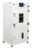
Cyanoacrylate Fuming Chamber w/water filtration
